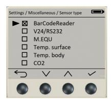
Depending on the selection of the sensor type, a pT symbol or an M symbol appears in the display of function button 1. This function button can also be used as an action/measurement trigger in addition to the red trigger buttons.
